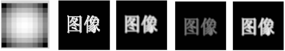
(a)模糊算子 (b)原始图像 (c)模糊图像 (d)原算法复原结果 (e)改进算法复原结果 (a) Blur operator (b) Original image (c) Degraded image (d) Restored image of original algorithm (e) Restored image of improved algorithm
